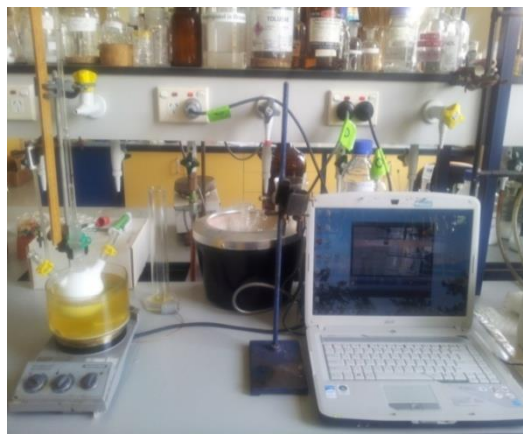
Figure(2): Photograph of watching the seeded emulsion polymerization of P( methyl methacrylate) with P-methyl styrene and two different surfactant.
