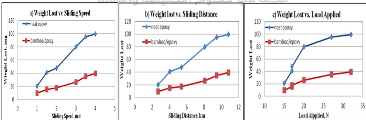
**Fig2.4: The relationship between weight lost and sliding distance, sliding speed and applied load(NE).**
