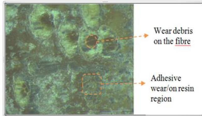
Fig.3.5. Illustrated the effect of high operational parameters.
