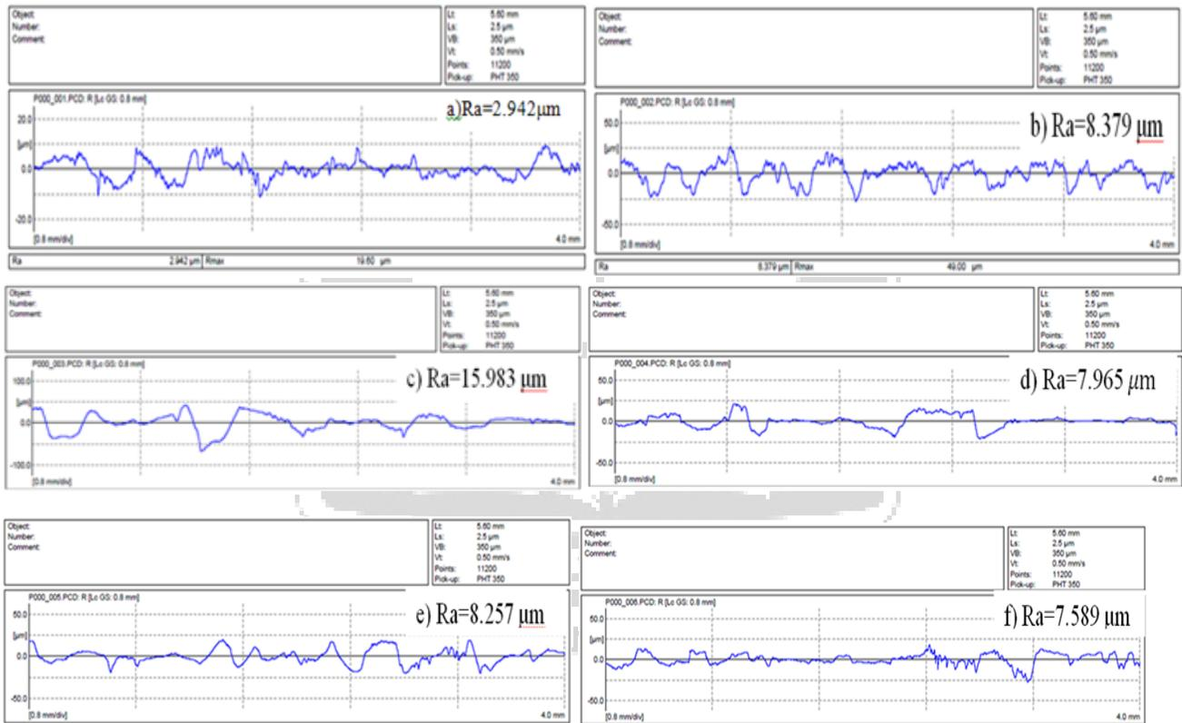
**Fig.4.2: The roughness profile of bamboo fibre reinforced epoxy.**
