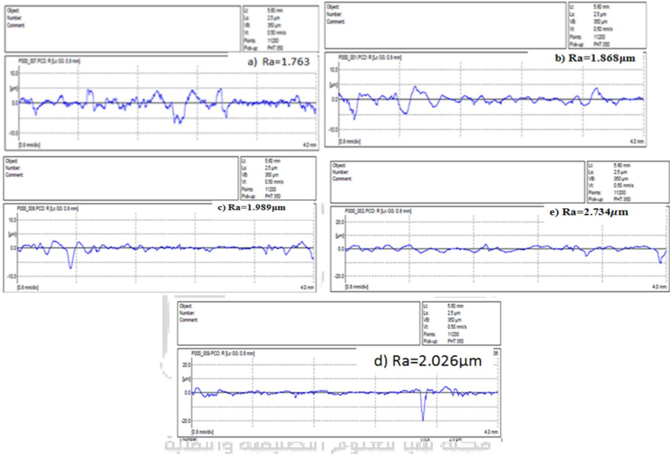
Fig.4.1: The roughness values of NE samples.
