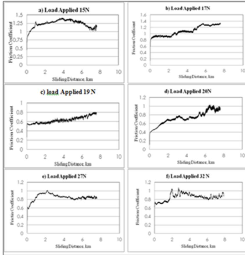
Fig.2.6. The frictional coefficient of neat epoxy
