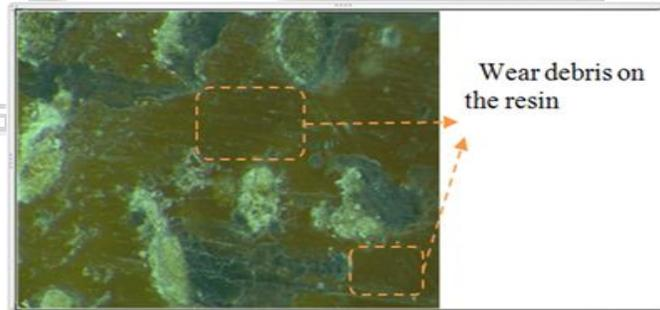
**Fig.3.4. The effect of high sliding velocity and high applied load.**
