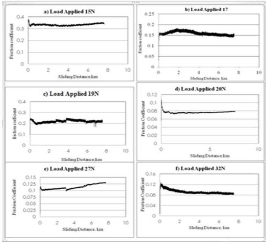
Fig.2.7. The frictional coefficient of bamboo reinforced epoxy.
