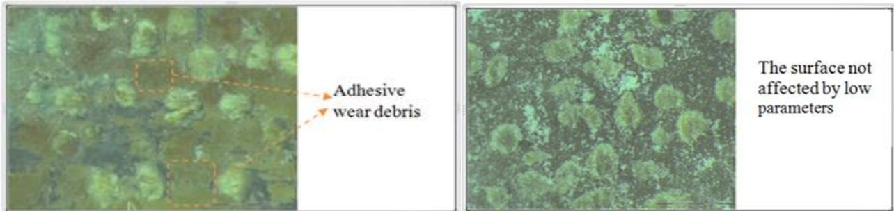
**Fig.3.2 Show the effect of low sliding distance operational and low applied load**
