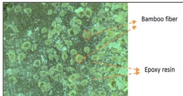
Fig.3.1 The distribution of fiber through the epoxy resin
