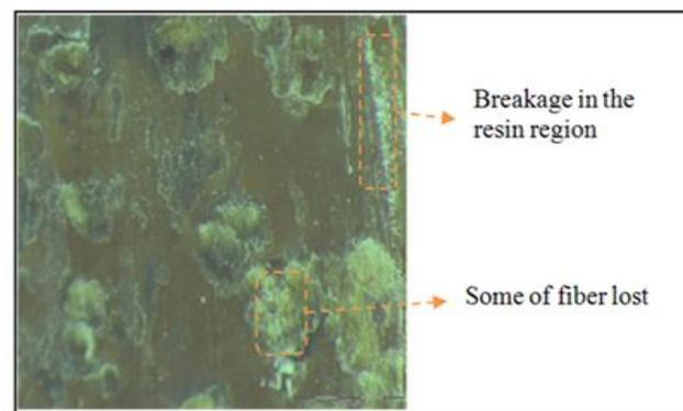
Fig.3.6. The effect of high operational parameters.
