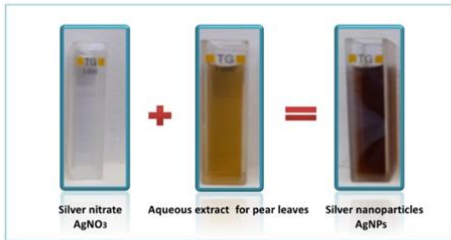
Fig.1 Color change due to AgNPs formation
